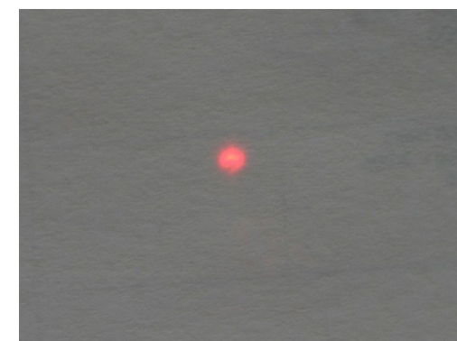
Figure 5: 633-nm diode laser aiming beam of the 10,600-nm CO 2 laser
