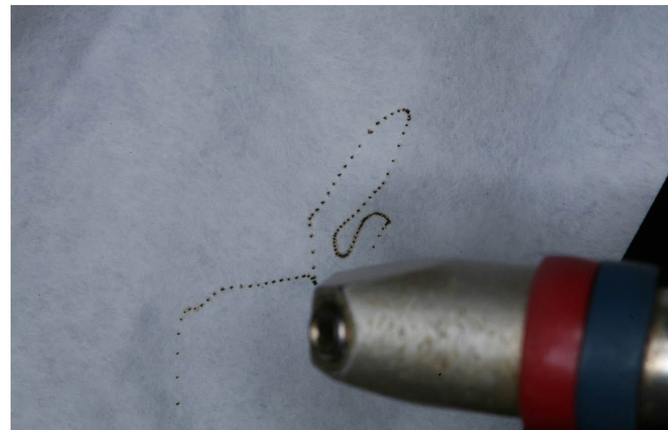
Figure 6: CO 2 laser test-fire on moist paper to detect appropriate interaction at low setting
